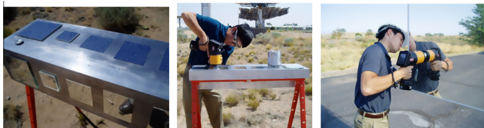
Fig. 2. Left: mirror samples affixed to sawhorse. Middle: measuring reflectivity of samples on sawhorse. Right: measuring reflectivity of heliostat facets.
