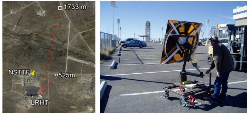
Fig. 5. Left: Map showing the locations of the single-facet beam tests at 525 m and 1733 m away from the long-range heliostat target (LRHT). Right: Rig used to hold and track the facets.
