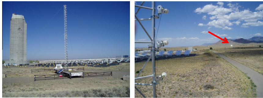
Fig. 6. Left: Long-range heliostat target (LRHT) Sment et al., 2012. Right: View from the (LRHT) looking at the solar reflection from a single facet \sim 1700 m away.
