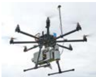
Figure 6c (left). Eight-engine unmanned aerial vehicle (UAV).
