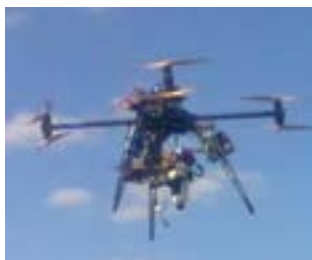
Figure 6c (left). Eight-engine unmanned aerial vehicle (UAV).
