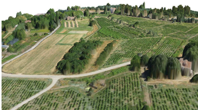
Figure 17. Digital surface model (DSM) of a UTAD's vineyard determined in the post-processing stage of a flight with an UAV carrying an optical sensor.
