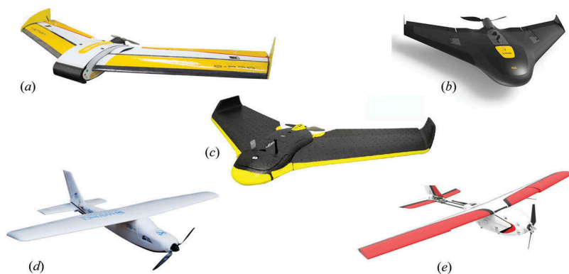
Figure 3. Some of the most representative fixed-wing UAVs: (a) QuestUAV Q-Pod; (b) SenseFly eBee; (c) Trimble UX5; (d) MAVinci Sirius Pro; and (e) PrecisionHawk Lancaster. The images were obtained from the manufacturers' websites.
