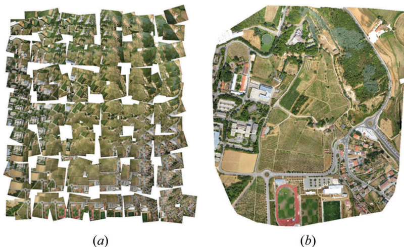
Figure 15. Ortophomoaig generation example. (a) Images gathered in a UAV flight over UTAD's campus. (b) Orthorectified image mosaic which is the result of the processing operations (involving homographic corrections and stitching) upon the acquired images.
